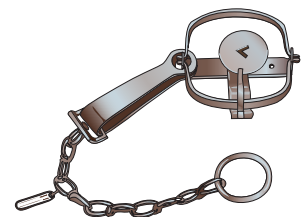
Foothold traps catch the animal when it steps on the trap.
